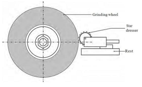
Dressing of a Grinding Wheel (Star wheel method)
