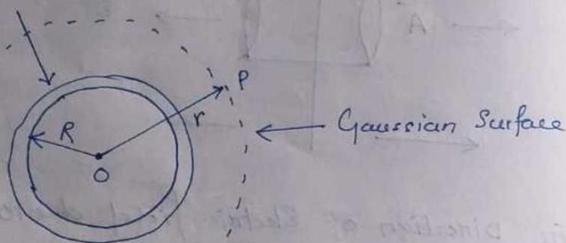
Electric field outside the spherical shell
