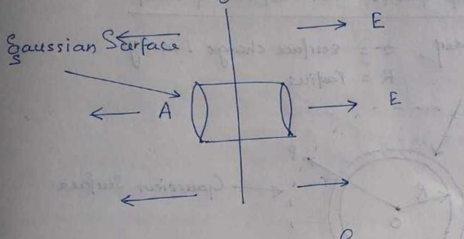
The direction of electric field due to an infinite charge sheet is perpendicular to the plane of the sheet.
