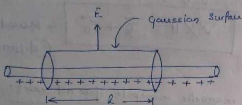
Let us consider an infinitely long wire with linear charge density ' $\lambda$ ' and length  $L$ . To calculate electric field, assume a cylindrical gaussian surface. electric field  $\vec{E}$  is radial in direction, the flux through the end of the cylindrical surface will be zero.
