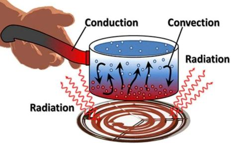
2) Convection: is the mode of heat transfer between a solid surface and the adjacent liquid or gas which is in motion, and it involves the combined effects of conduction and fluid motion.
