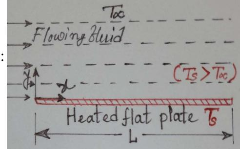
figure where a fluid flows having temperature  $T_{\infty}$  over the heated plate at temperature  $T_s$ .
