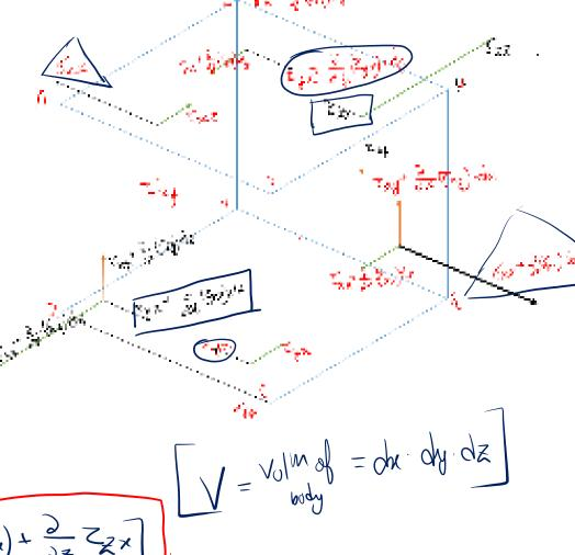
$$F_{R} + F_{V_{x}} = \frac{\partial}{\partial x} \left( S_{xx} \right) \cdot V + \frac{\partial}{\partial y} \left( Z_{yx} \right) \cdot V + \frac{\partial}{\partial z} \left( Z_{zx} \right) \cdot V$$
