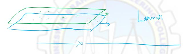
Laminar flow tollows Newton's Law of vis co sity
