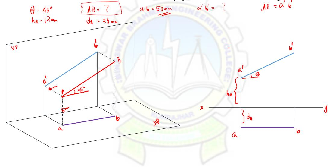
Q.3 The length of the top view of a line parallel to VP and inclined at 45 degree to HP is 50 mm. One end of the line is 12 mm above HP and 25 mm in front of VP. Draw the projection and determine the true length of the line.
