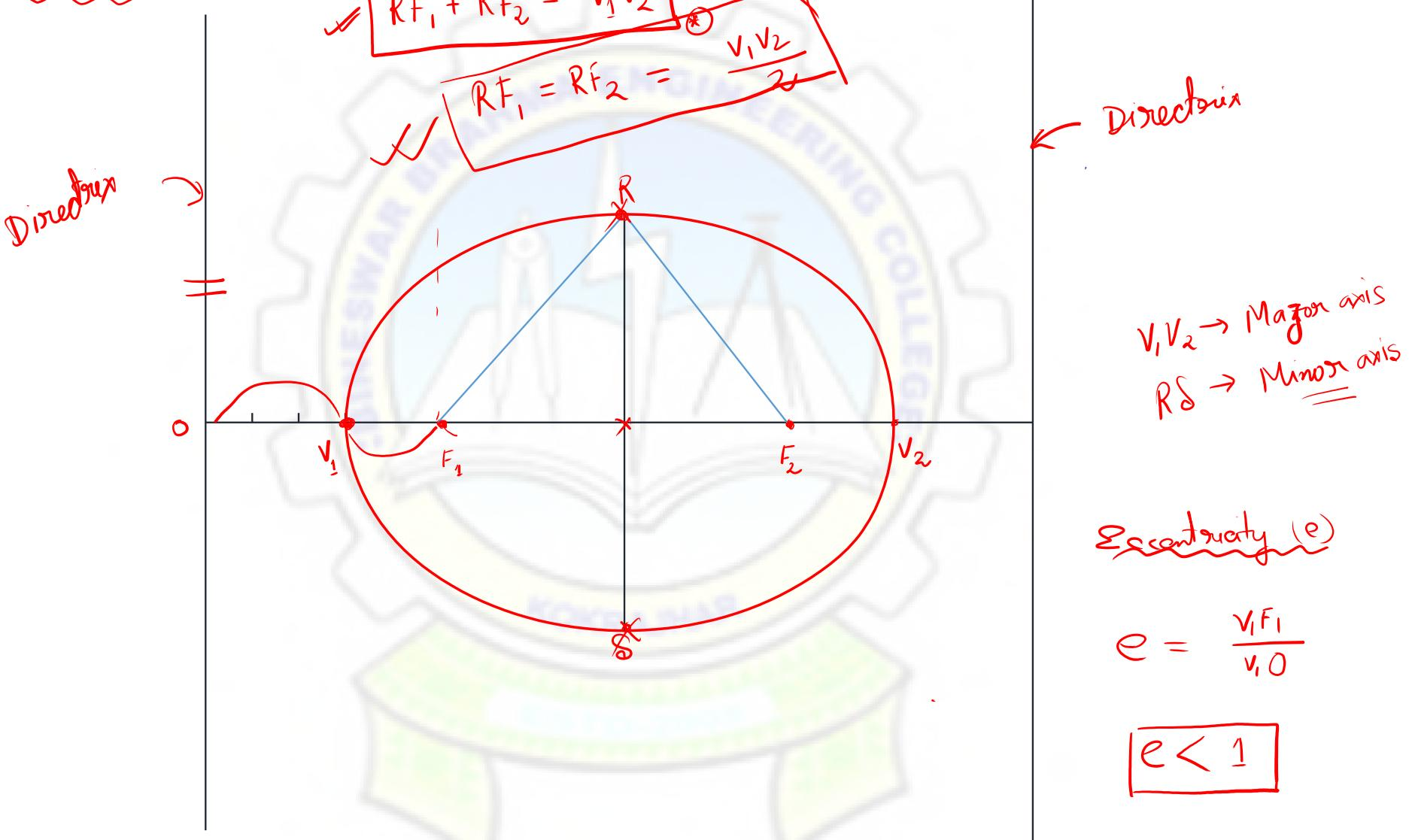
1/④ Construct an ellipse whose eccentricity is  $\frac{2}{3}$  and the distance of the directrix from focus is 50 mm.
