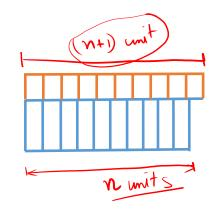
Q. 1 Draw a vernier scale of R.F. =  $\frac{1}{25}$  to read c.m. and long enough to measure upto 5 meters.
