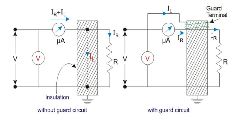
In the first circuit the micro ammeter measures both capacitive and the resistive current leading to error in value of R, while in the other circuit the micro ammeter reads only the resistive current.
