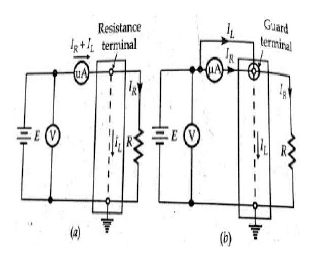
The **direct deflection method** is that of the figure-(b) above. For high resistance, such as insulation resistance of cables, a sensitive galvanometer of d'Arsonval type (usually having a current sensitivity of at 1000 mm/µA at a scale distance of 1 metre) is used in place of the microammeter. In fact, many sensitive types of galvanometers can detect currents from 0.1 - 1 nA. Therefore, with an applied voltage of 1 kV, resistances as high as 10^12 to 10\*10^12 can be measured.
