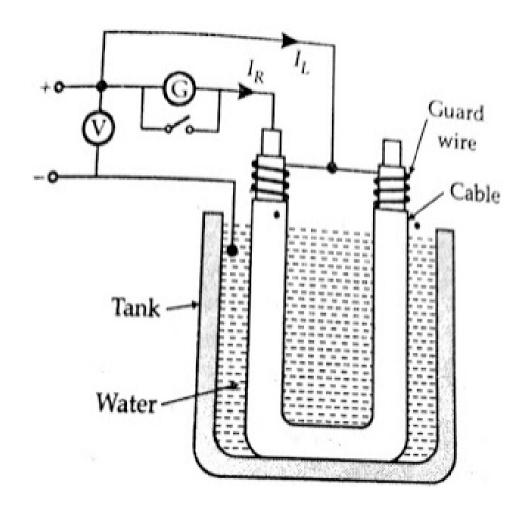
In some cases, the deflection of the galvanometer is observed, and its scale is afterwards calibrated by replacing the insulation by a standard high resistance (usually 1 MO), the galvanometer shunt being varied, as required to the adeflection of the same order as before.
