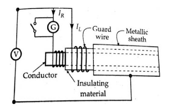
Cables without metal sheaths can be tested in a similar way if cable, except the end or ends on which corrections are made, is immersed in water in a tank. The water and the tank then form the return path for the current. The cable is immersed in slightly saline water for about 24 hours, and the temperature is kept constant (at about 20°C) and then the measurement is taken as in the figure below.
