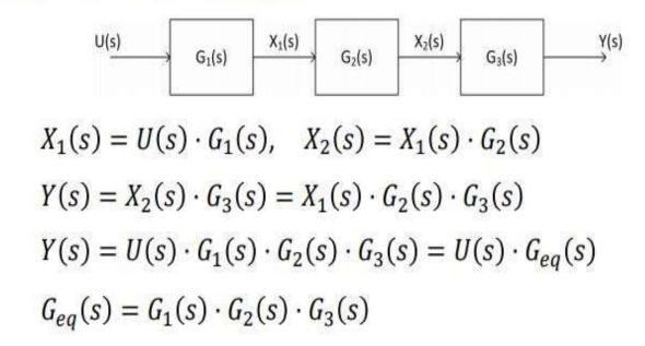
The equivalent transfer function of cascaded blocks is the product of the individual transfer functions
