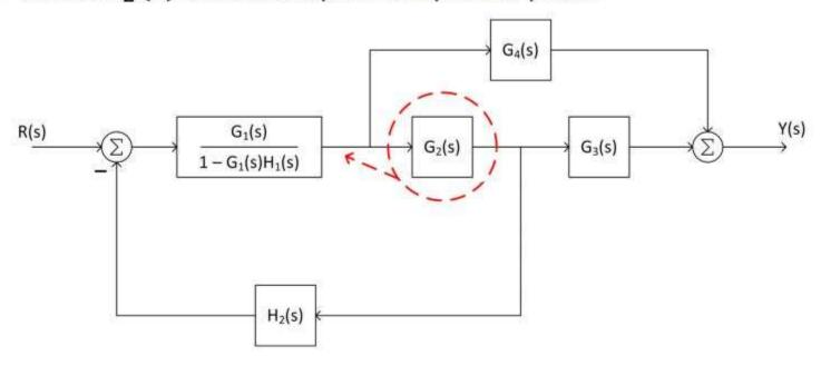
Block from previous step,  $G_2(s)$ , and  $H_2(s)$  become a feedback system that can be simplified
