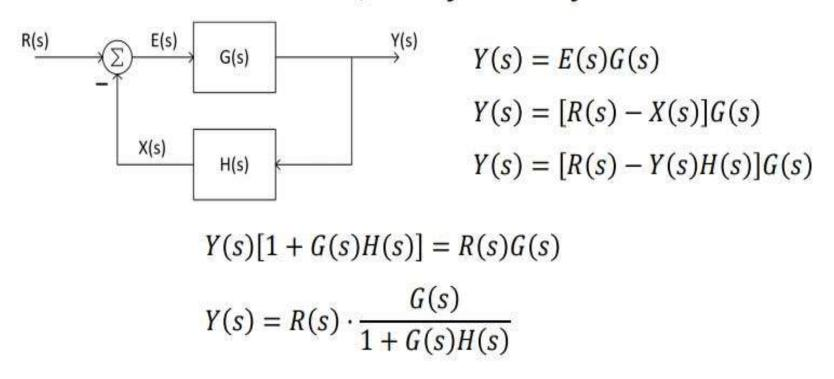
$\square$  The **closed-loop transfer function**, T(s), is
