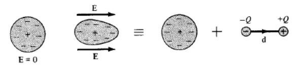
A dipole results from the displacement of charges and the dielectric is polarized. In polarized the electron cloud is distorted by the applied electric field.
