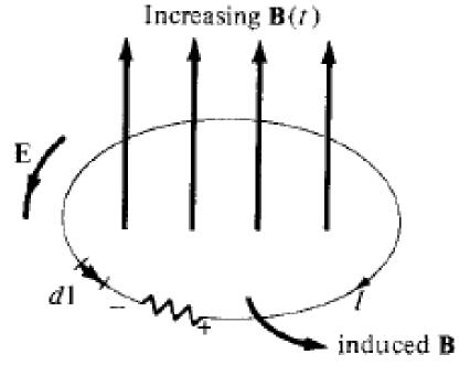
This emf induced by the time-varying current in a stationary loop is often referred to as transformer emf in power analysis since it is due to the transformer action.
