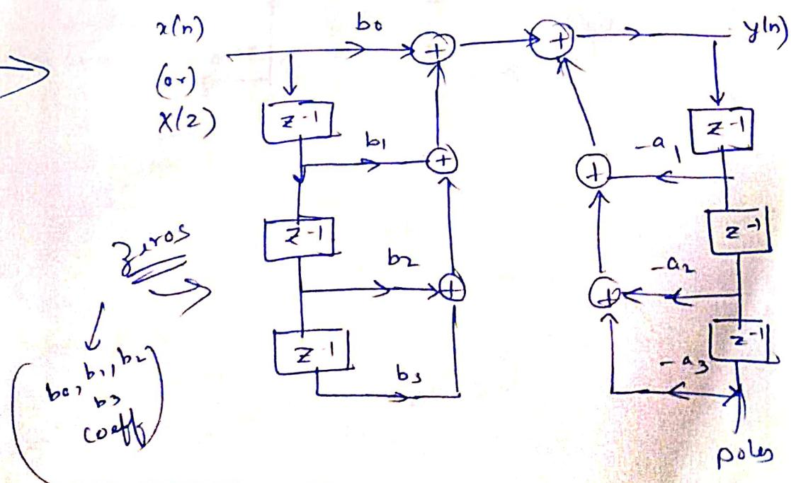
Ex: Determine <sup>direct</sup> Form I & Form II realizations for a third order IIR Transfer functions:
