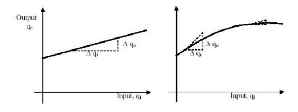
$$Sensitivity = \frac{Infinitesimal change in output}{Infinitesimal change in input}$$
