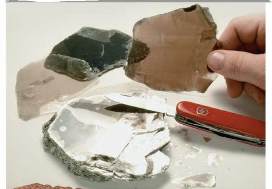
FIGURE 2.15 The thin sheets shown here were produced by splitting a mica (muscovite) crystal parallel to its perfect cleavage. (Photo by Chip Clark)
