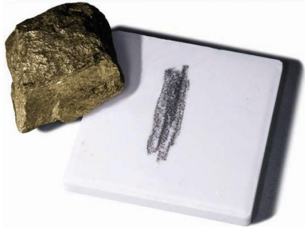
FIGURE 2.11 Although the color of a mineral is not always helpful in identification, the streak, which is the color of the powdered mineral, can be very useful. (Photo by Dennis Tasa)
