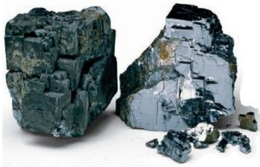
FIGURE 2.9 The freshly broken sample of galena (right) displays a metallic luster, while the sample on the left is tarnished and has a submetallic luster. (Photo courtesy of E. J. Tarbuck)
