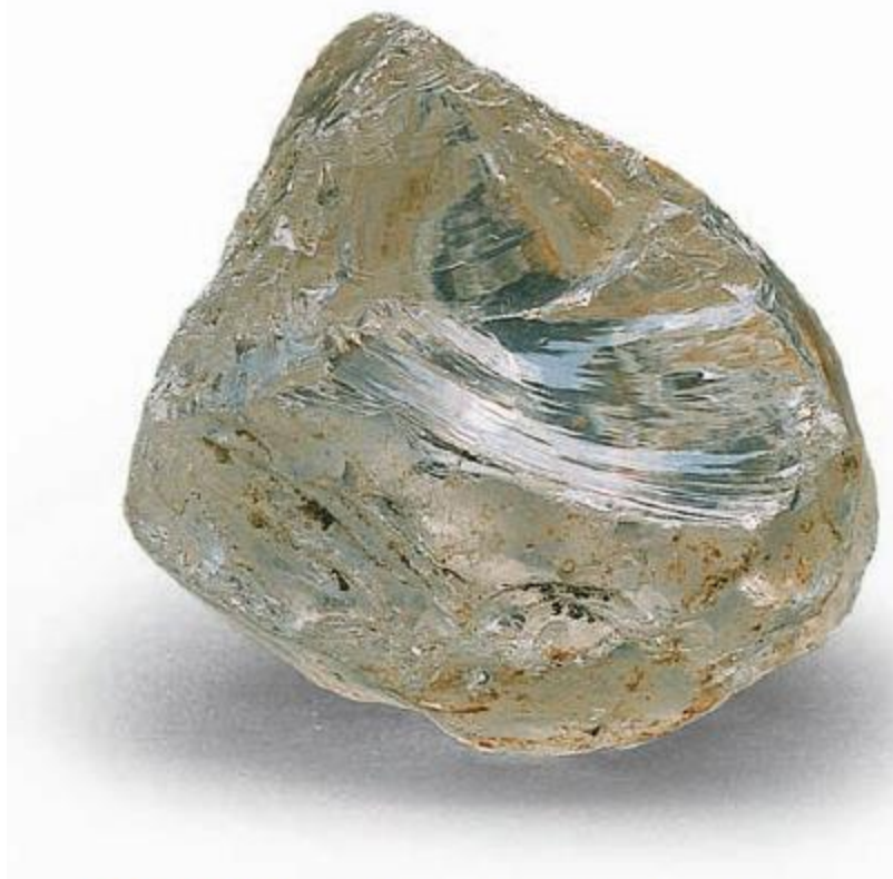
FIGURE 2.17 Conchoidal fracture. The smooth curved surfaces result when minerals break in a glasslike manner. (Photo by E. J. Tarbuck)
